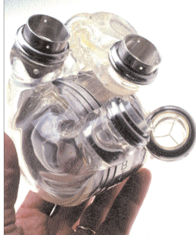
The AbioCor is a titanium and plastic electric-powered heart that, unlike previous devices, fits in the chest with no wires or tubes poking through the skin. It works with a small external battery pack that transmits power to an internal coil.
