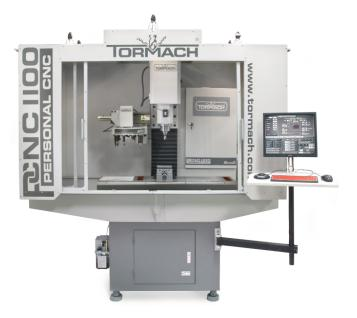
**Tormach PCNC 1100 mill** Four axis. Work envelope 18"x9.5"x16.25". 1100W 1.5HP spindle. PathPilot control. For high-density materials that need rigid tooling and flood coolant. Steel, aluminum, brass, iron, titanium.
