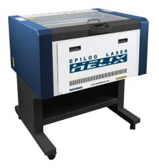
**2 Epilog Helix laser engravers** Bed size 24"x18". One 75W, the other 80W. A rotary attachment is available for cylindrical objects. Cuts medium and light density materials such as acrylic, wood, paper, cardboard. Can engrave glass, stone, anodized aluminum, painted steel.
