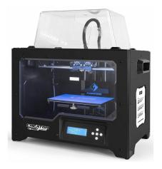
**FlashForge Creator MAX** Dual-extrusion FDM. 225xx145x150mm build volume. 1.75mm filament. Full enclosure makes it suitable for ABS.
