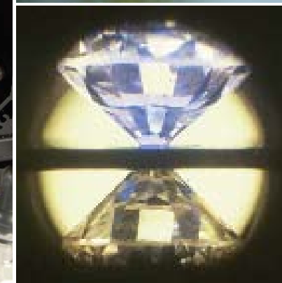
All in a day's work: Hemley examines diamonds made by chemical vapor deposition in the adjacent chamber. (Center top): gem-quality diamonds from the lab; (bottom) a diamond anvil cell; (right) a 12 mm long diamond single crystal from the lab.
